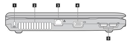
**1 Kensington slot** Attach a security lock (not supplied) here.
